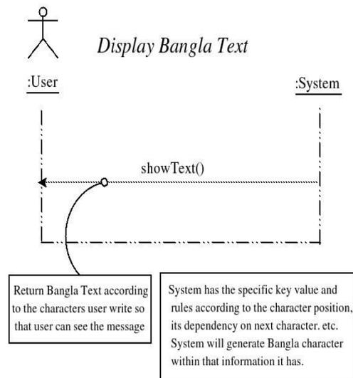
Figure 3b: System Sequence diagram of the use case - Display Bangla text
