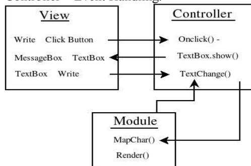
Figure 5: Model View Controller of the system
